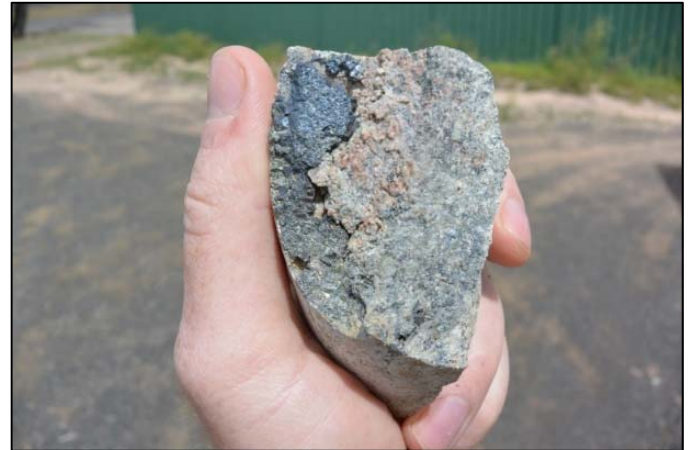
Figure 2. Chalcocite mineralisation within fractures and veinlets of the supergene enriched copper zone at Coalstoun copper deposit
